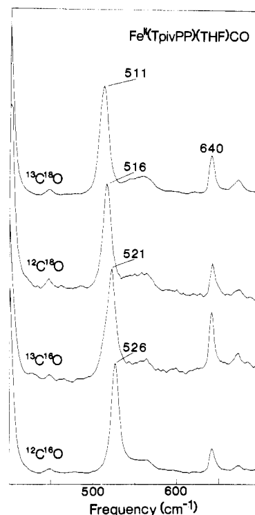
FIGURE 4: Carbon monoxide isotope effects on the low-frequency region (400–700- \text{cm}^{-1} ) spectra of \text{Fe}^{\text{II}}(\text{TpivPP})(\text{THF})(\text{CO}) . \lambda_{\text{exc}} = 406.7 \text{ nm} ; concentration 50 \mu\text{M} . Neat THF solution.
